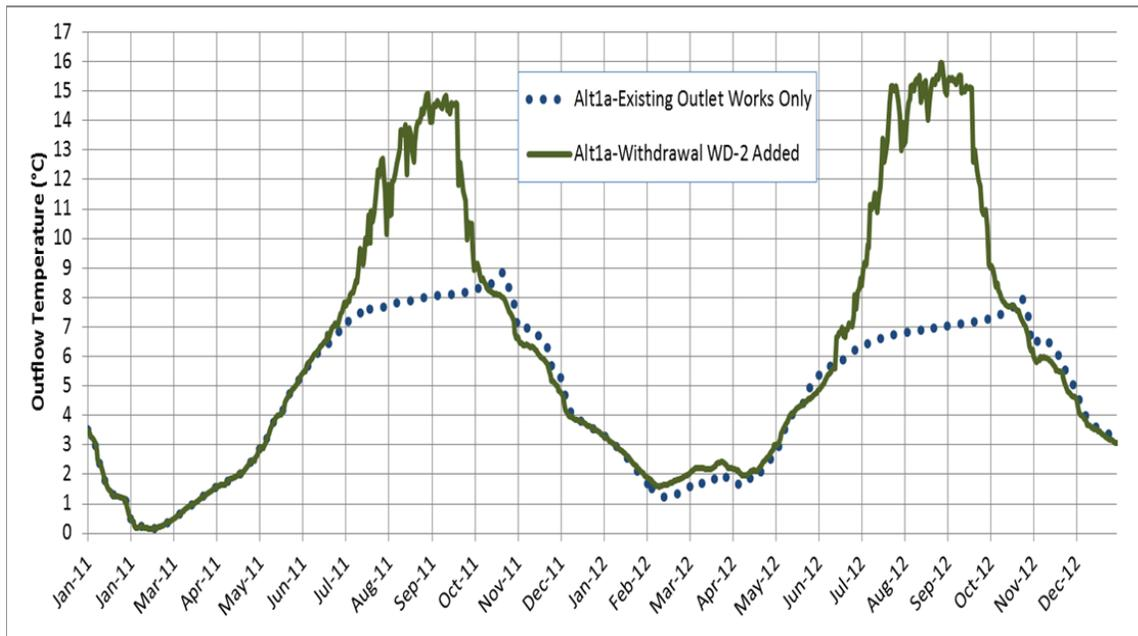
Figure 4. Simulated Gross Reservoir Outflow Temperatures for Alt1a With and Without Selective Withdrawal. From 2013 Hydros Draft Memo: “DRAFT Results of Preliminary Model Run of Selective Withdrawal in Gross Reservoir”
