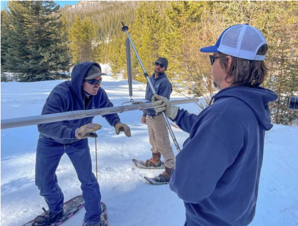
Denver Water employees calculate the density of a snow sample collected near Winter Park on April 28, 2022. The samples are used to assess how much water is in the mountain snowpack.
